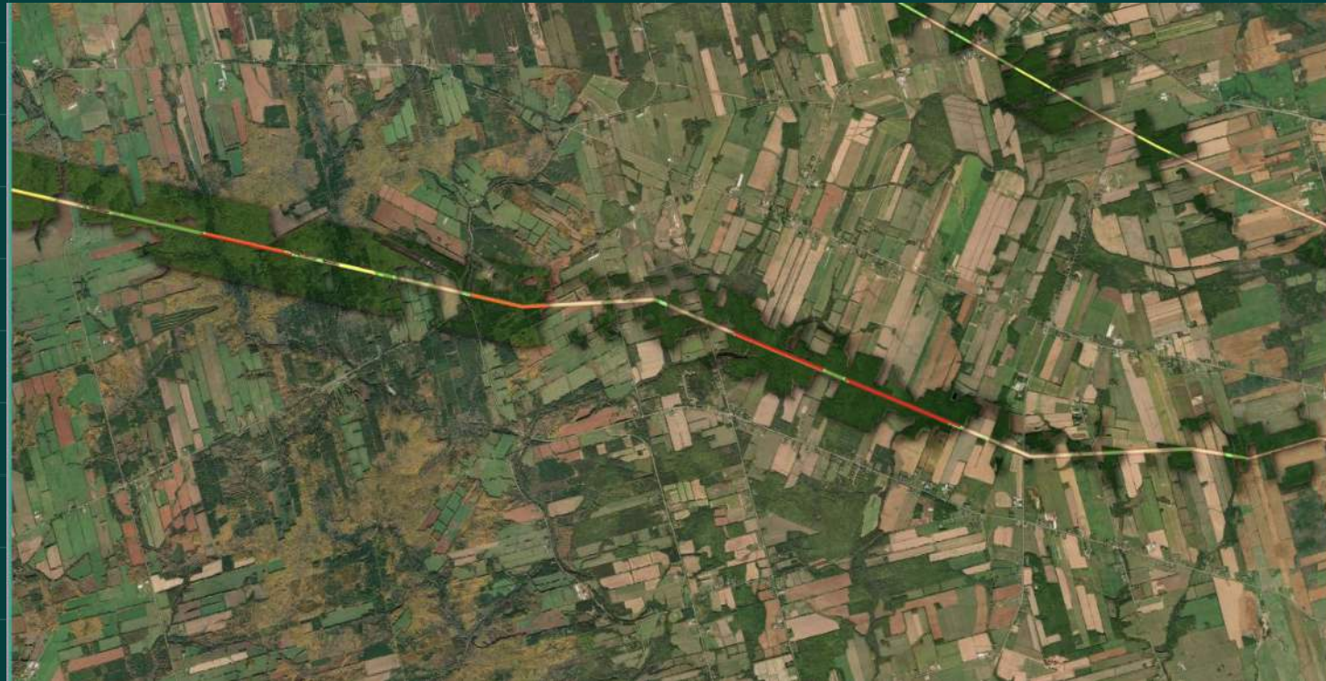
Dark green polygons indicate densely forested areas, with colour indexed markers identifying risk level to power lines.
