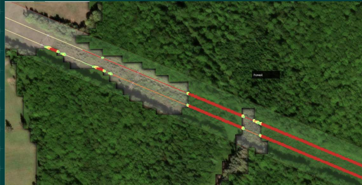
Close up of a stretch of the transmission network span, with indications of at-risk locations posed by vegetation in close proximity to power lines. These span analytics indicate an action for proactive risk mitigation.
