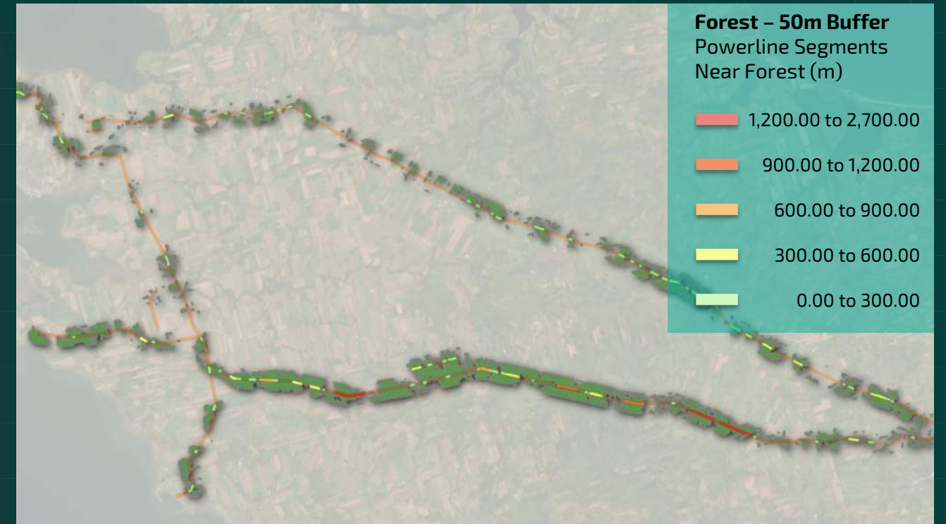
Network categorized by proximity to vegetation, with red highlights indicating high risk areas with Right-of-Way or ROW proximity less than 50m from power lines.
