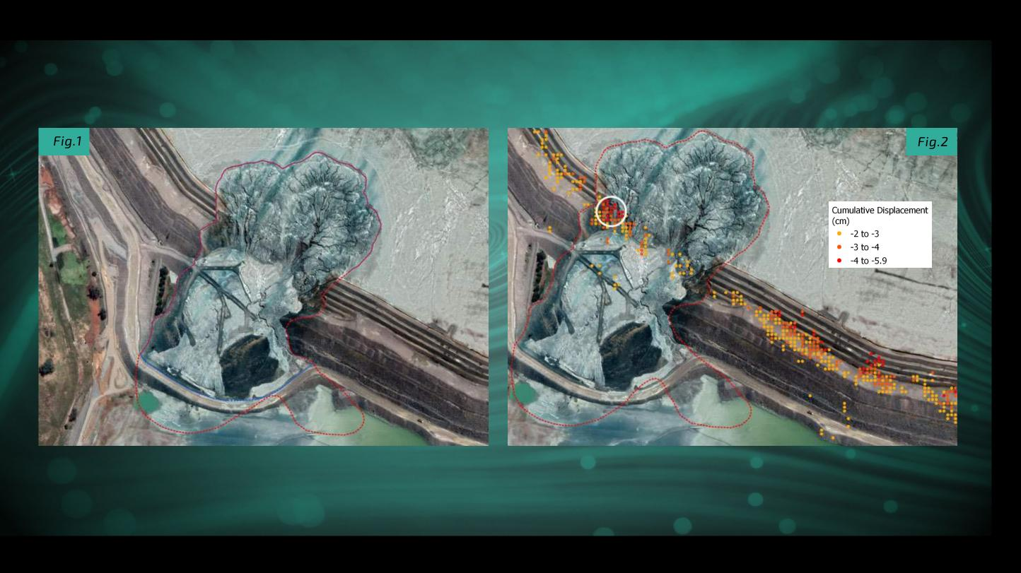
Combining satellite imagery of the breach with historical InSAR analysis, our team identified several areas of negative ground displacement spanning the length of the wall at the point of failure.
