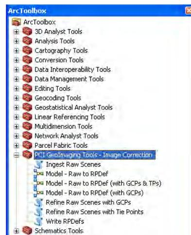
▲ Figure 1 - GeoImaging Tools for ArcGIS GUI integrated in ArcGIS
