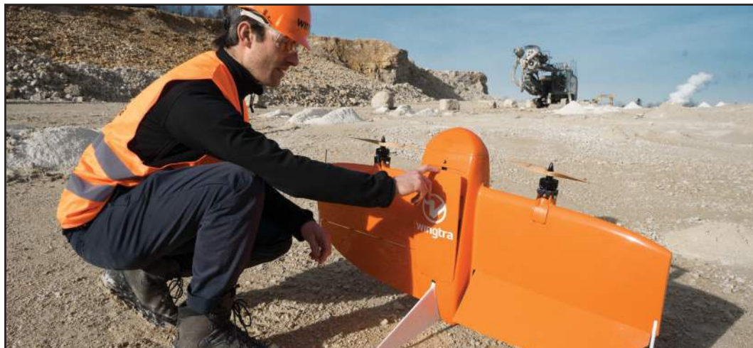
Vertical take-off and landing (VTOL) capability allows the WingtraOne to move like a helicopter.
