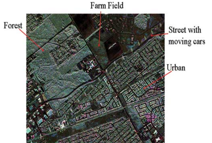
Fig. 5. Convair-580 multipolarization SAR image (Ottawa, ON, Canada). (Red) HH. (Green) HV. (Blue) VV.
