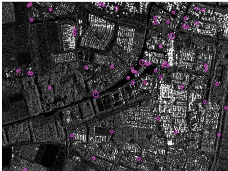
Figure 7: Change detection using point target heuristics
