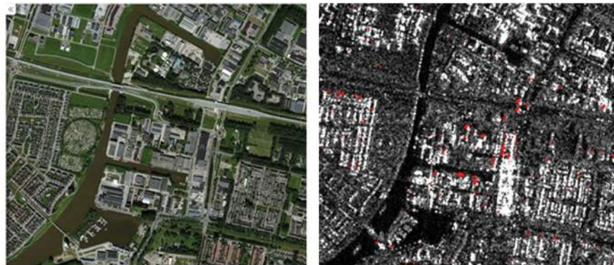
Figure 12: Flevoland optical image (Bing Maps™) and RADARSAT-2/TerraSAR-X point target change map
