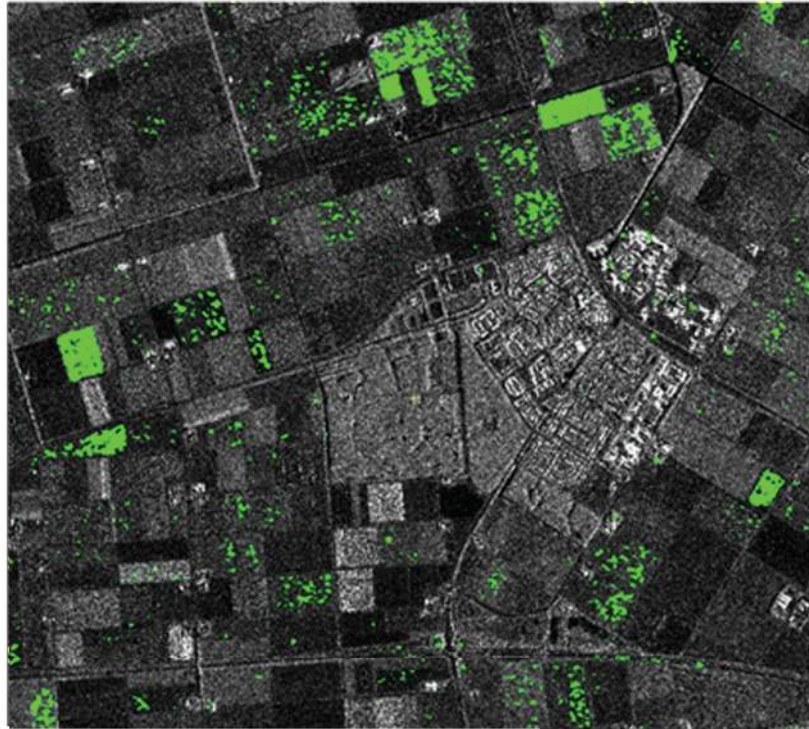
Figure 4: Top 2% of changes detected by CCDWISH
