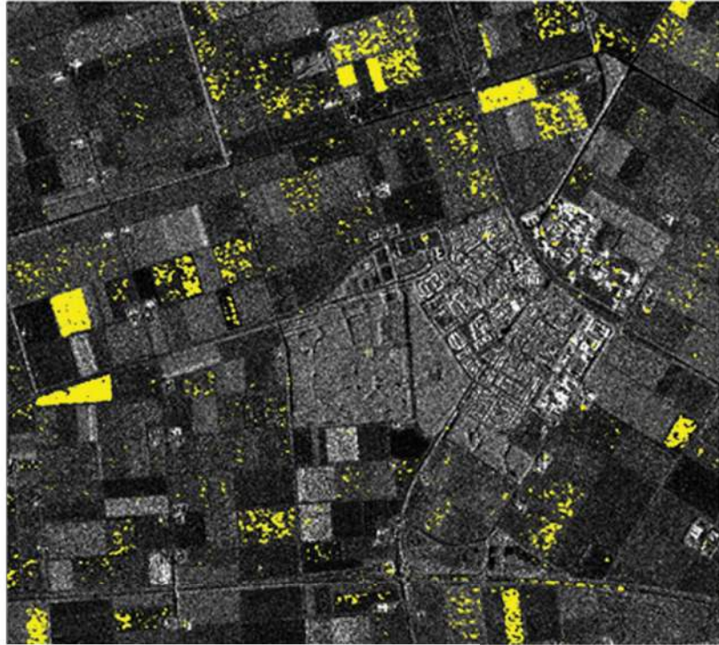
Figure 2: Top 2% of changes detected by CCDINTEN
