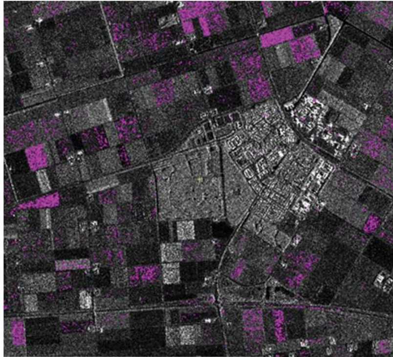
Figure 5: Top 2% of changes detected using results from CCDINTEN, CCDPHASE and CCDWISH
