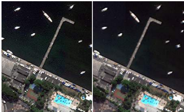
Pansharpener: Non-Pansharpener (left), Pansharpener (right) improving quality (Imagery Credit: Maxar).
