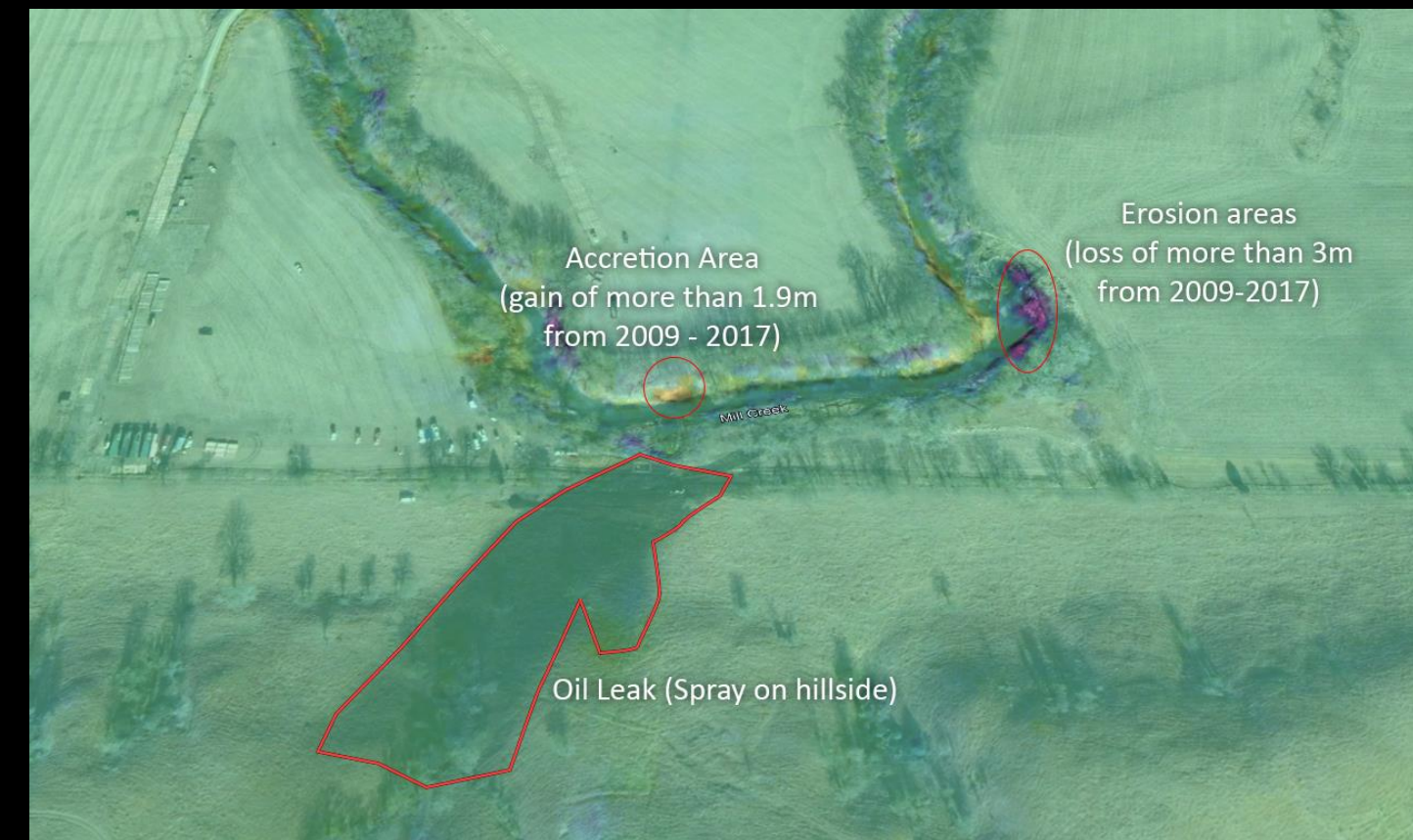
Figure 2: A recently collected satellite image (Credit Maxar) is shown with elevation change analysis carried out by CATALYST.
